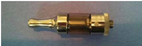
Figure 6: Tank that holds the wick and liquid components of e-cigarette
